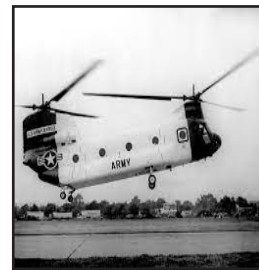
Sept. 21, 1961: The first fully equipped U.S. Army Chinook designated the CH-47A completed its first flight. The Boeing Chinook is one of the world’s most reliable and efficient transport helicopters, capable of handling loads up to 28,000 pounds with a maximum gross weight of 54,000 pounds.
