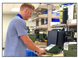
appropriately. Lab technicians calibrate these machines, which are used to test gas masks for leaks prior to deployments or field exercises for units from every branch in the military.
