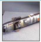
June 29, 1993: U.S. Army Materiel Command approved the release of the AGM-114F Interim Helicopter Launched Fire and Forget Missile, or Hellfire, for use with the AH-64 "Apache" attack helicopter. The interim missile had a new warhead section containing a second (forward) warhead, which allowed the system to defeat contemporary fielded reactive armor.
