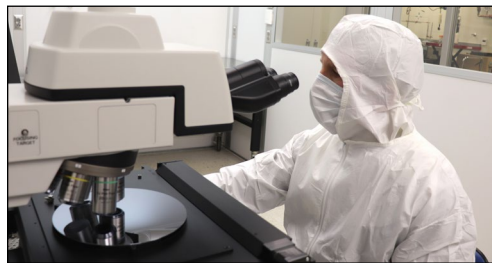
Miles Owen, a USATA metrologist with the Army Primary Standards Laboratory, counts aerosol particles deposited onto a silicon wafer in the APSL clean room.
