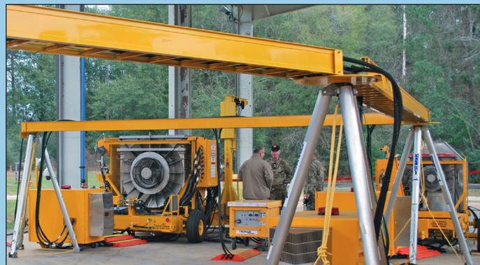
The Army's first Modernized Flexible Engine Diagnostic System (MFEDS) (ACLC photo)
