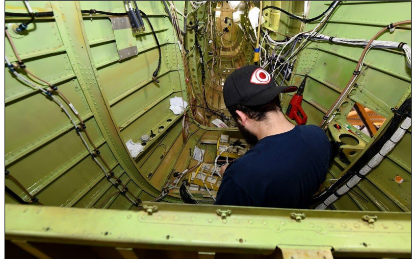
John Farhat, aircraft electrical mechanic III with Amentum, at the Corpus Christi Army Depot, Texas, installs arc 220 wiring for the UH-60L communications system inside the aircraft tail section. This is the first aircraft (8BZ32) to be painted using 100% class N (non-chromate) primers on the interior and exterior.
